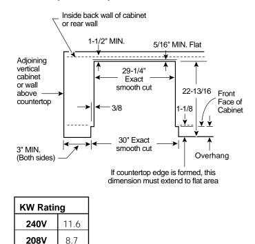
**Important:** 30" Drop-In Ranges are designed to hang from the countertop. It does not rest on the floor. For installation alternatives, refer to installation instructions packed with product.
